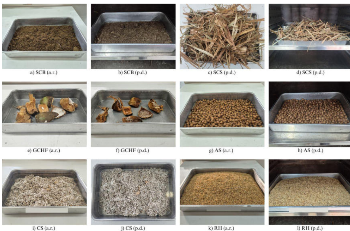
Fig. 2. Raw biomasses (AS, CS, GCHFB, RH, SCB and SCS) as received (a.r.) and after pre-drying (p.d.) at (105 \pm 5) ^\circ\text{C} .
